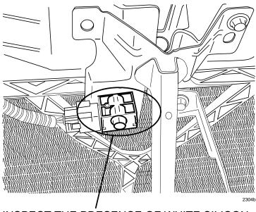
INSPECT THE PRESENCE OF WHITE SILICON AT BOLT HEAD, END OF BOLT, ON TOP OF, AND SURROUNDING SURFACES OF CRASH ZONE SENSOR
